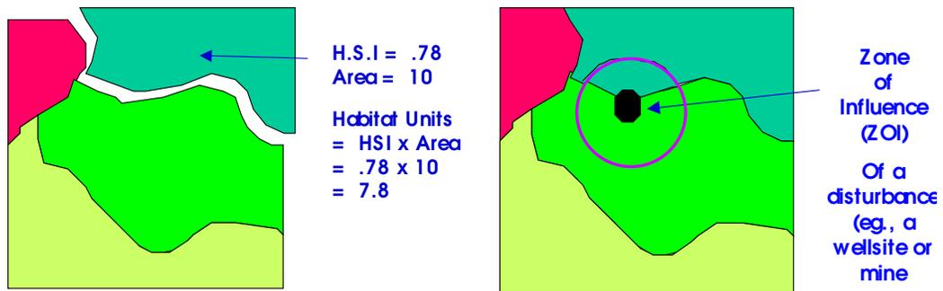
Note: Shaded areas are “polygons” in a GIS representing patches of contiguous vegetation, soils and terrain features as interpreted by an ELC.
